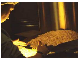
13. Capsules are sorted and visually inspected on specially designed R&D Inspection Stations
